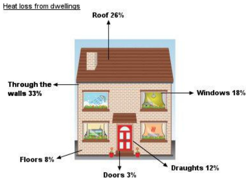
You can save up to 33% of your heating costs by wall insulation. There are several ways of insulating a solid or stone wall. Some similar methods can also be used for timber framed walls in older properties. This is best done when and if you plan to re-decorate.
